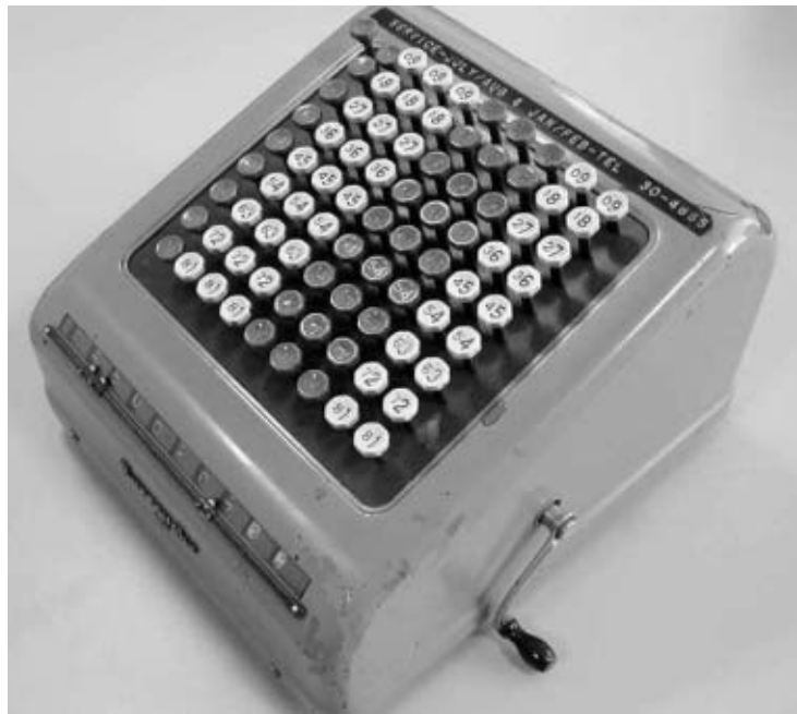
A comptometer – a mechanical adding machine as used in the Audit Office from the 1920s to the 1960s.
