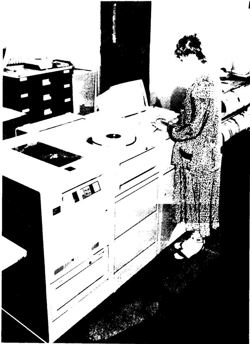
The VAX 8350 minicomputer: the centre of the Office's local area network.
