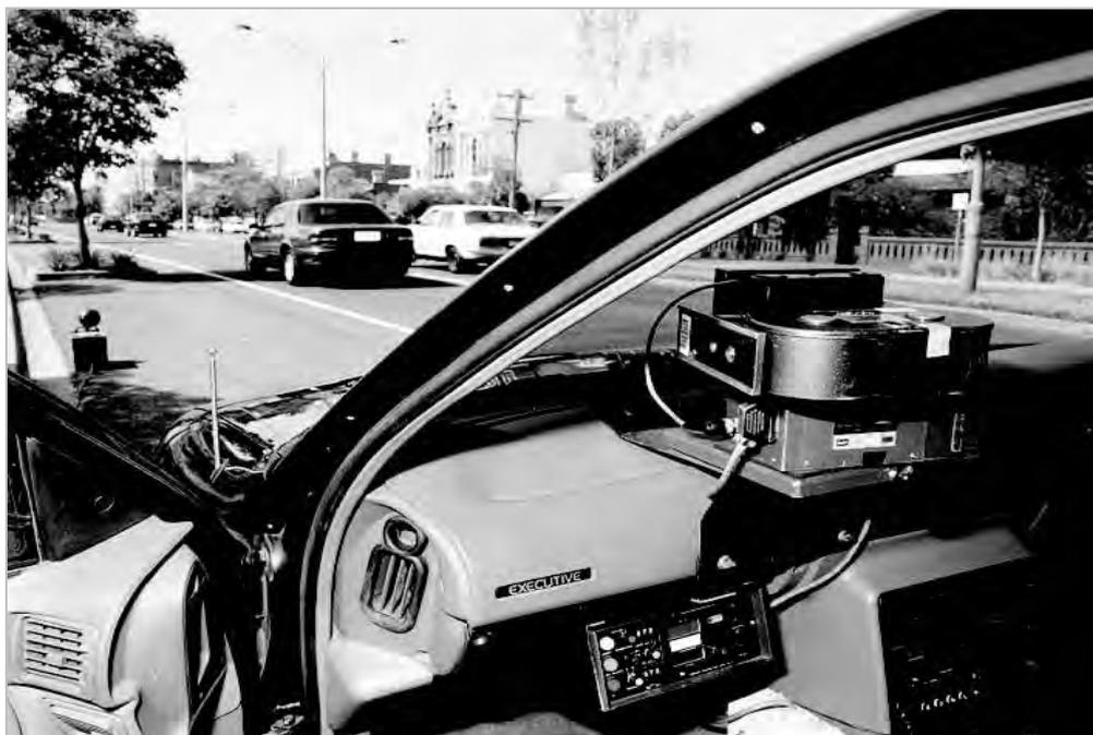
*A mobile speed camera mounted inside a mobile camera car. (Photo courtesy of the Department of Justice.)*
