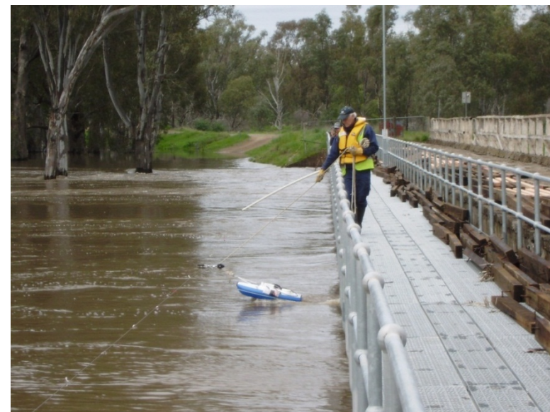
Flood monitoring with acoustic doppler on the Goulburn River at Loch Garry. Photo courtesy of DEPI.
