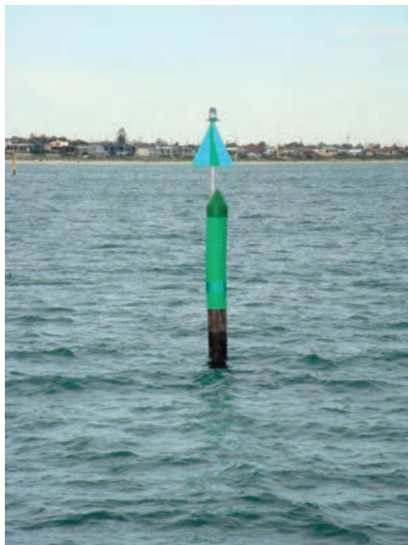
Starboard mark near Mordialloc Pier marking the entrance to Mordialloc Creek. Note special mark in the background delineating 5 knot zone.
