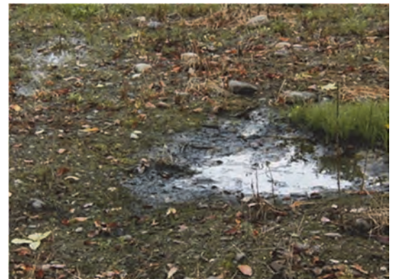
Pooling of domestic wastewater from failing onsite system. Photo: South East Water.
