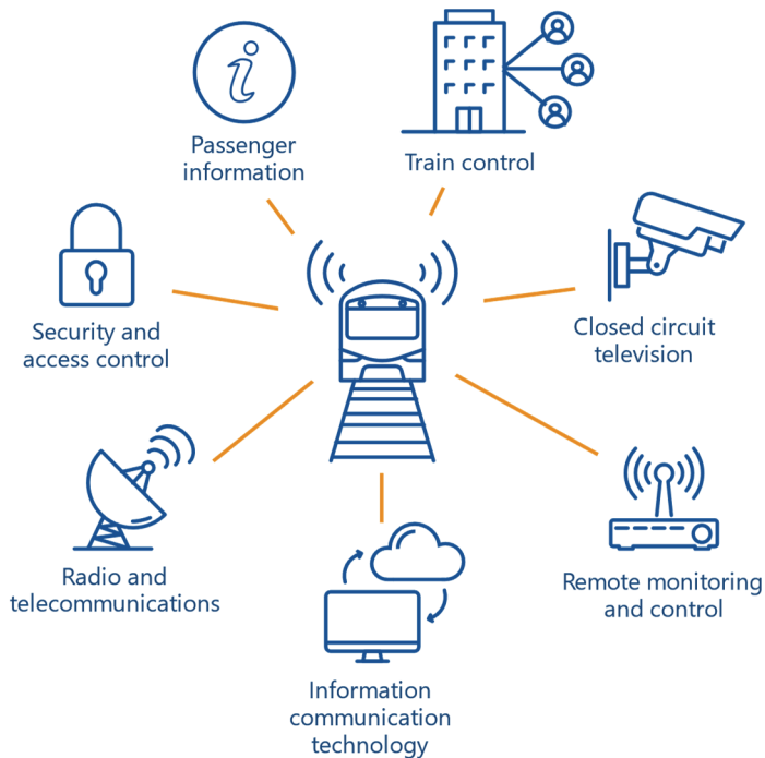
Figure 1F: Technology assets on railways
